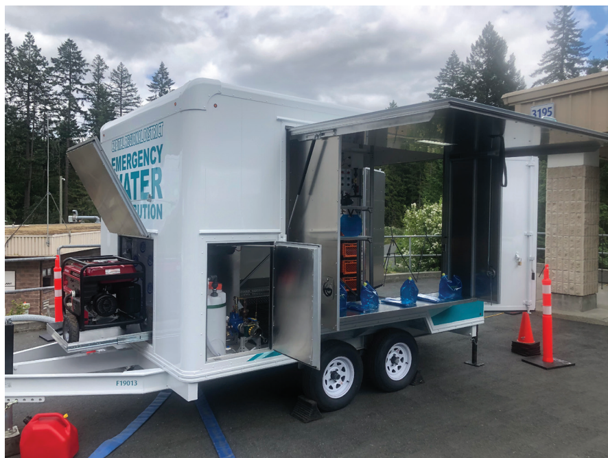
The CRD's new emergency water distribution units are self-contained, location deployable mobile water distribution stations designed to dispense drinking water to the public during an emergency.
