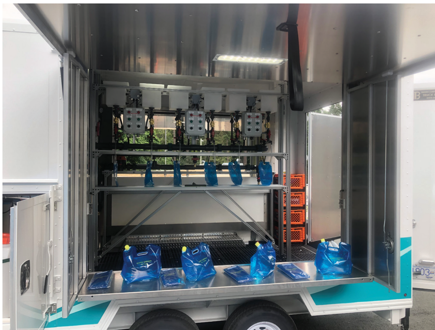
The public-access sides of the EWDUs are designed to accommodate public “bag fill,” featuring multiple push-button/auto shut-off spigot stations dispensing precisely five litres of water.
