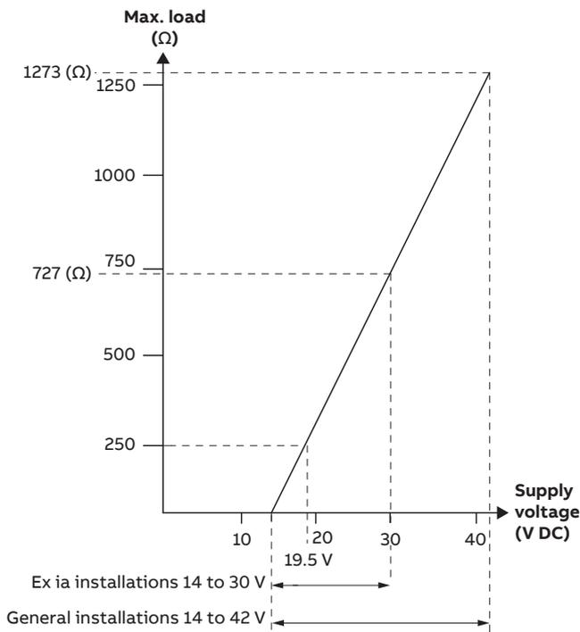
With 250 Ω resistor for HART communication min. supply voltage = 19.5 V DC
