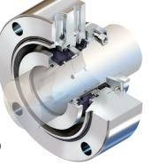
A single cartridge seal in a flexible stator design with rugged primary seal faces of sintered silicon carbide in a monoblock configuration. Available with a Quench Containment Device (QCD) as an outboard seal that can be run with a low pressure water closed loop barrier system or as a single seal with the Synthetic Lubrication Device (SLD) that requires no other equipment.
