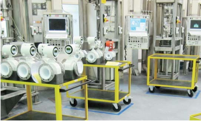
Calibration facilities for fluids with (5-350) m 3 /h
