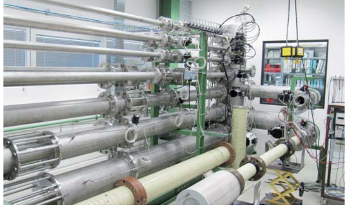
Calibration facilities for gases with (1-8.800) kg/h
