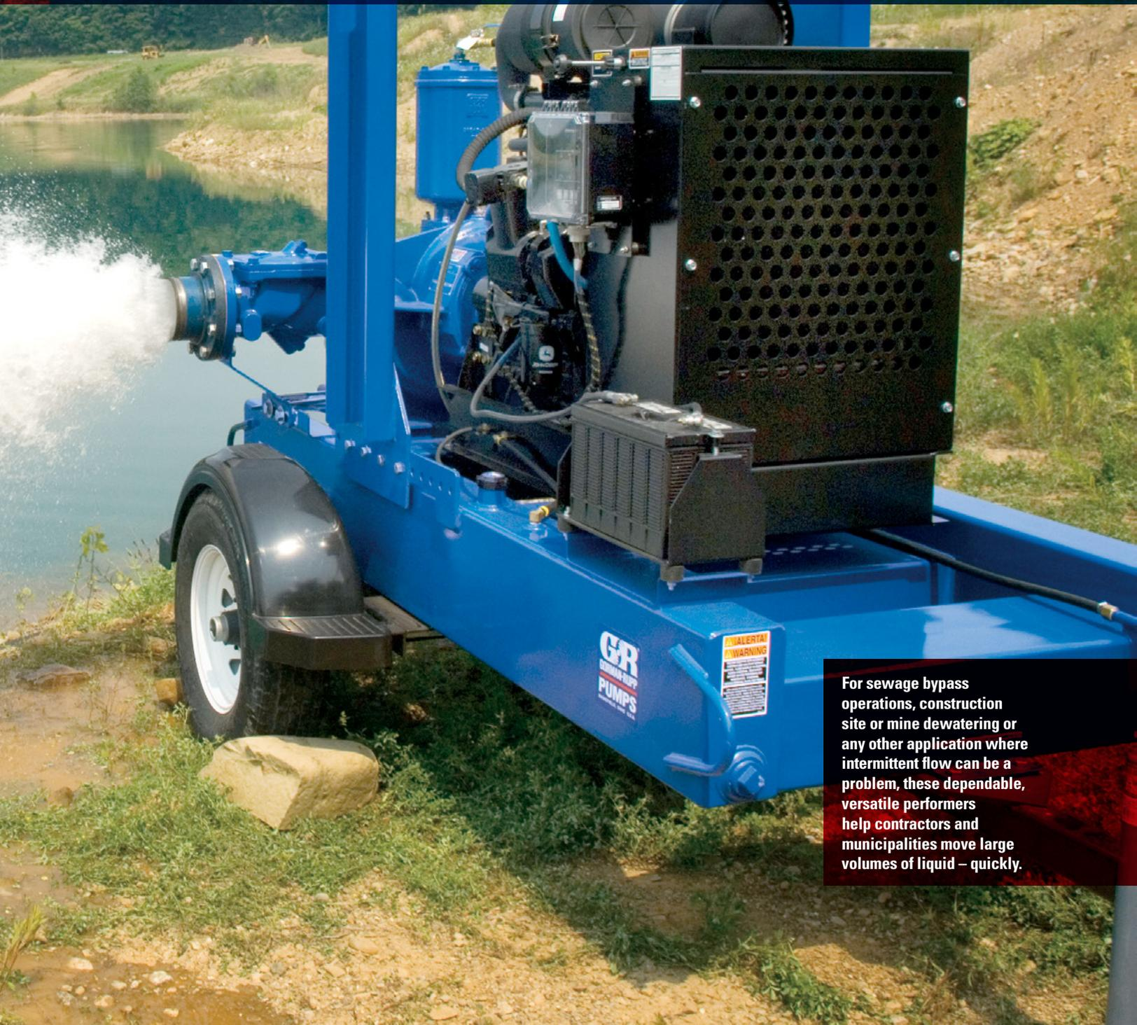
For sewage bypass operations, construction site or mine dewatering or any other application where intermittent flow can be a problem, these dependable, versatile performers help contractors and municipalities move large volumes of liquid – quickly.
