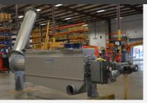
The Whitetip Shark Washing Compactor features screenings drainage and compaction zones. Stainless steel flights and antirotation bars improve compaction and provide reliable equipment performance and life.
